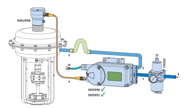
Figure 12. TYPICAL APPLICATION, CODE W
