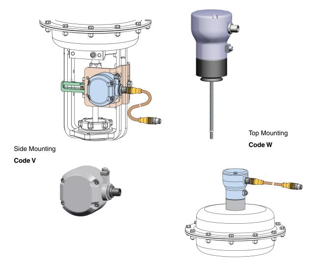
The RMU998 Remote Mounting Unit is the solution for valve/actuator applications in harsh environments, such as operating the valve at very low or very high temperatures and high vibrations. The position of the actuator is determined by an external potentiometer in the RMU998 and transmitted to the positioner which is mounted in a protected environment.
